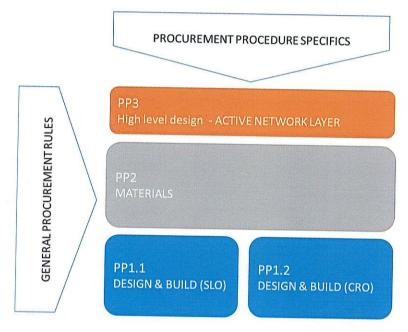
PP1.1 and PP1.2 procedures are aimed at the design and construction of the passive layer of the future network. Both contain designing and building of the infrastructure and include all permission gathering, in a way to reduce the operative risk deriving from the differences between the plan and the effective situation on the field.
